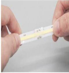
After complete the insert, also make sure both ends of led strip are tightly connected.
