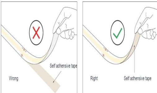
If the led strip needs to be torn up, please make sure that the self adhesive tape is torn with the led strip, otherwise the led strip will be damaged.
